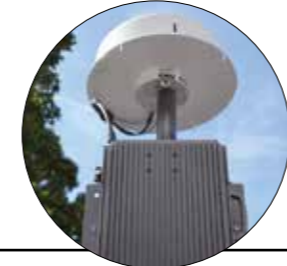
STATION CHARLIE (fixed installation): ▶ SignalShark Outdoor Unit ▶ ADFA ▶ LTE modem ▶ Software: Decodio ReX
