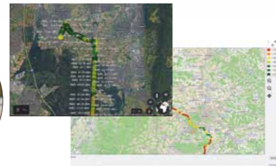
Script: Coverage Map The SignalShark synchronously records the level and position. These can be displayed as a coverage map on the internal map, or imported e.g. into Google Earth by exporting in *.kml format.
