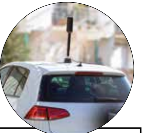
STATION ALPHA (mobile): ▶ SignalShark handheld ▶ Omnidirectional antenna ▶ LTE modem ▶ Software: Decodio ReX
