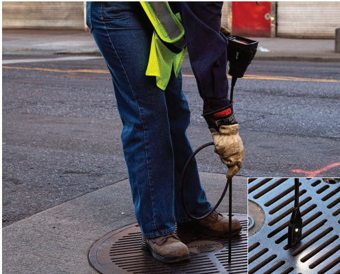
Figure 6.2 Insert the probe into the test area.
