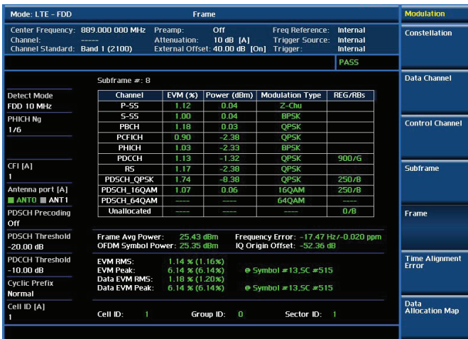
Modulation analysis — Frame
