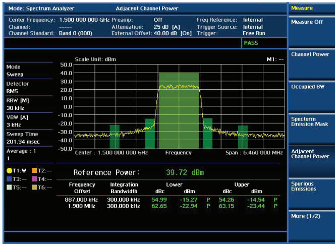
RF test — Adjacent Channel Power
