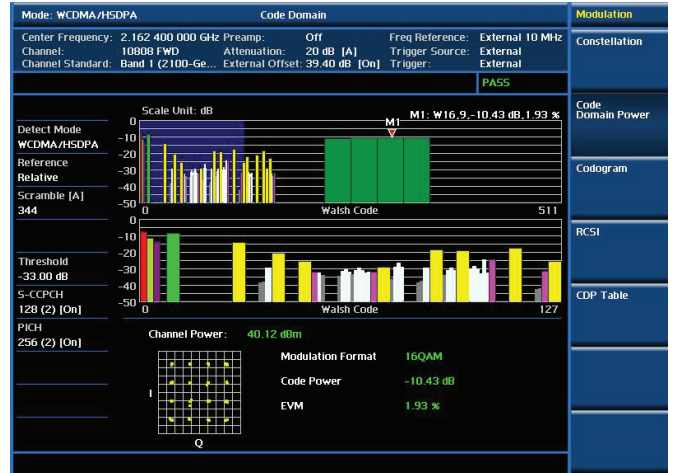
Modulation analysis — Code Domain Power
