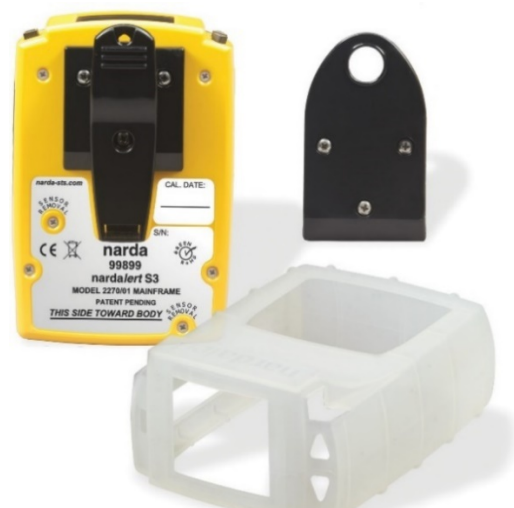
Fig. 3. Silicon rubber skin and interchangeable clips
