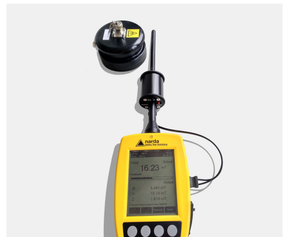
Figure 4: Measurement on a permanent magnet with operation via the NBM-550 measuring device
