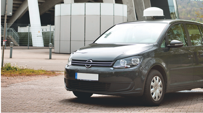
Fig. 3. Magnet mount – Non-destructive, fast mounting on a vehicle roof
