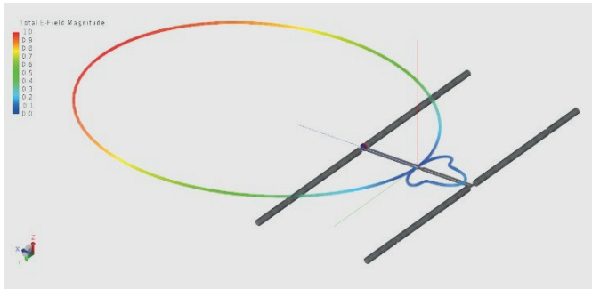
Fig. 10. Antenna 2 - Typical horizontal characteristic of the directional dipole antenna, computed for the far field.
