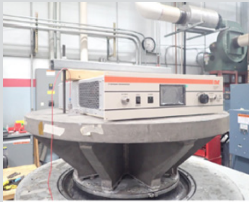
High power RF module: 1.4 kW peak min 1-400 MHz
