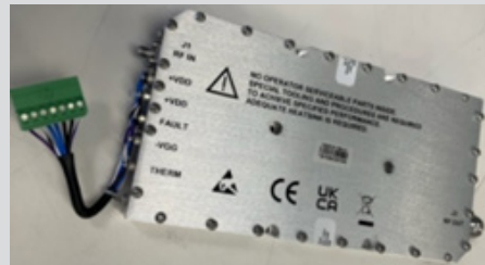
A Single RF Block Tested up to 40 G axes
